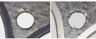
Worn, uneven cut tools to save cost. Poor sealing ability.
