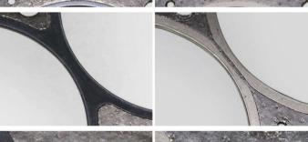
Separated fire rings to save tooling cost. Prone to compression leaks over-time.
