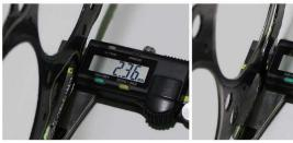
30% reduction in thickness to save material cost. Reduce engine service life.
